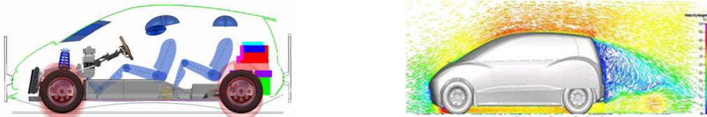
Figure 12: BEV packaging theme and aerodynamic study
