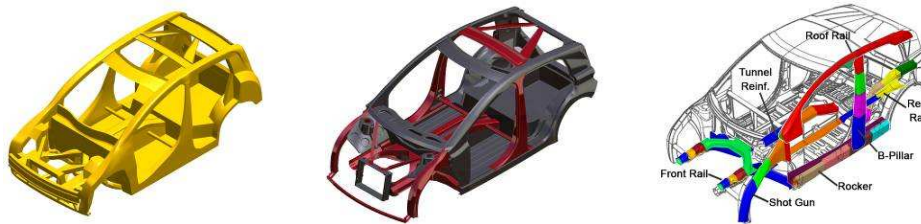
Figure 14: LF3G optimization, reference body structure and structural sub-systems
